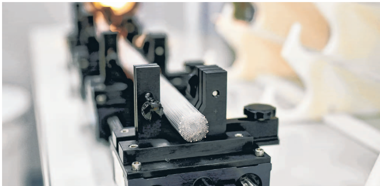
Small glass tubes known as core tubes in the OFS Hollow-Core lab at the beginning stage of hollow-core fiber fabrication.
